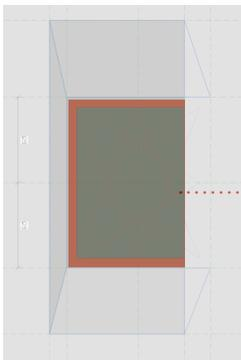
In window families where the opening is obstructed in elevation view, the visible projection shall be calculated as glazing area.
