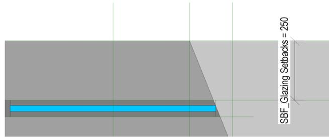
Use Parameter "SBF\_Glazing Setbacks" from shared parameter list for glazing offset from the Exterior side of the wall
