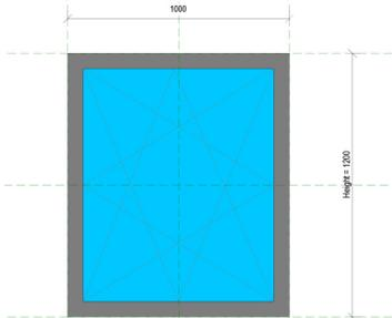
When modeling window and door families Built-in Parameters "Width" and "Height" should be used.
