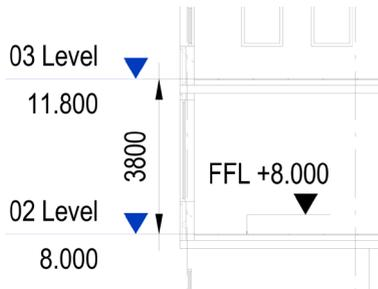
**Important note: Floor to floor height will be calculated from FFL level to FFL Level, so no floor offsets will be taken in consideration!**
