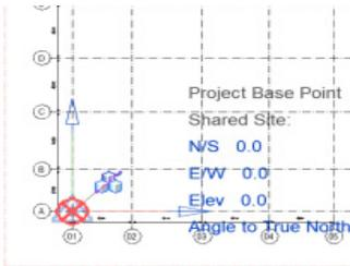
Project Base point must be clearly defined and visible on one of the administration views and positioned on the lower left grid intersection
